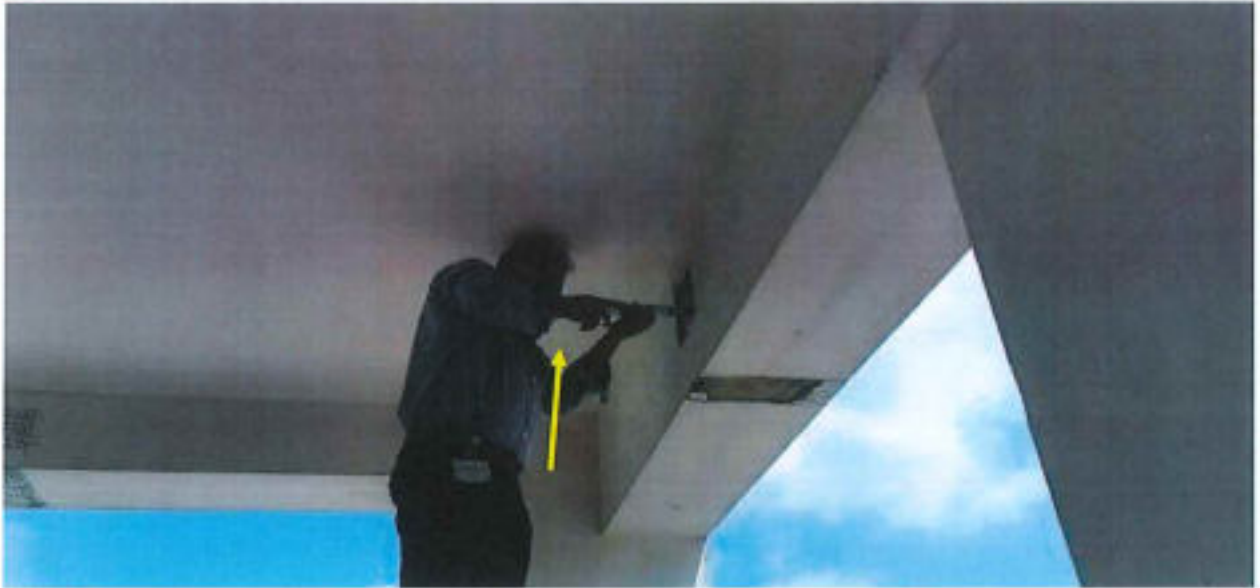
Rebound hammer test in progress (Typical view)
