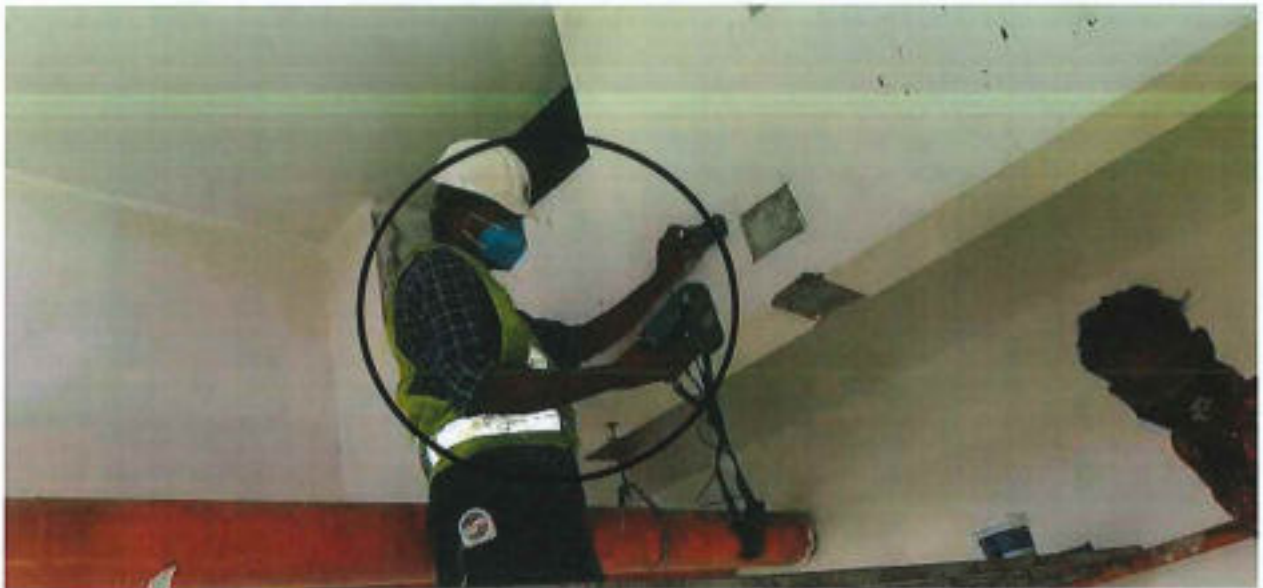
Cover meter test in progress (Typical view)
