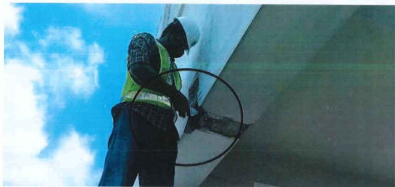
Carbonation test in progress (Typical view)
