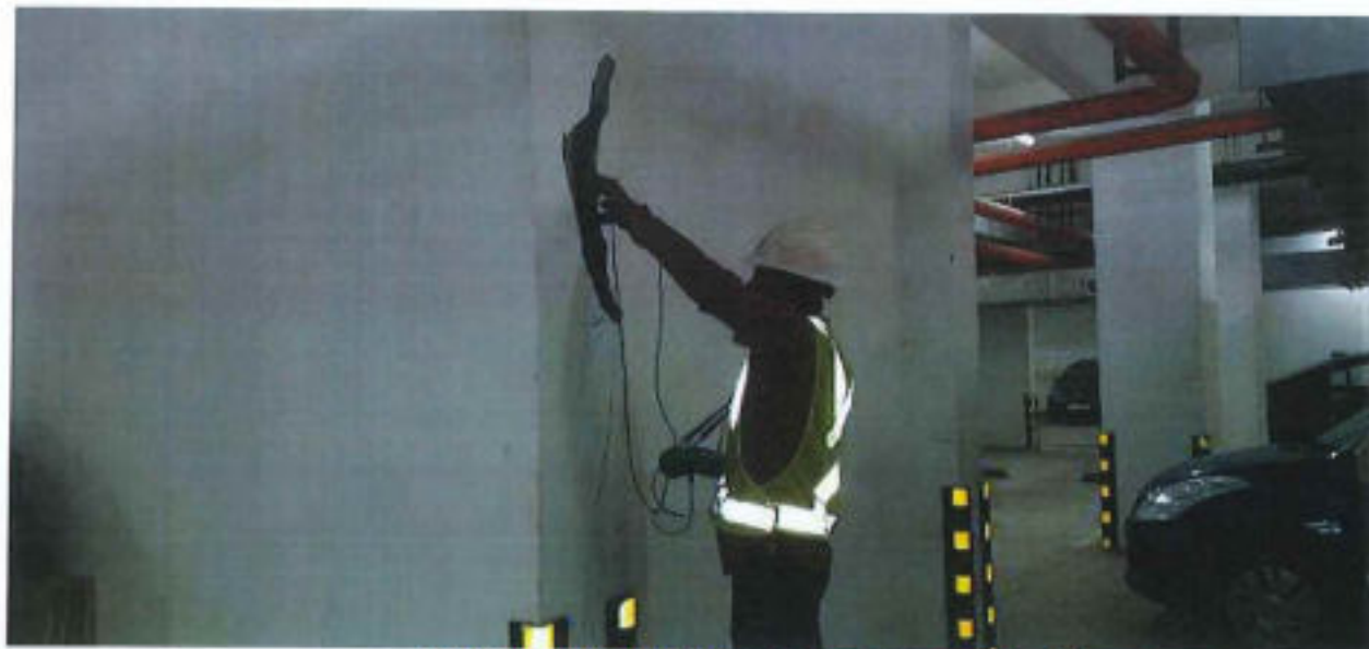
Half-cell potential difference measurement test in progress (Typical view)
