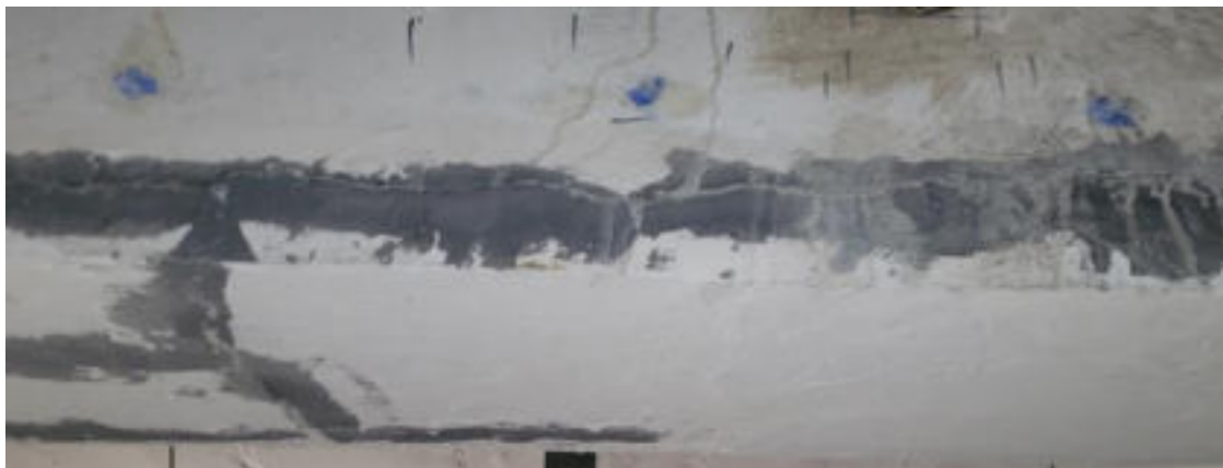
(e) Cracks reappeared in patch-repaired beam
