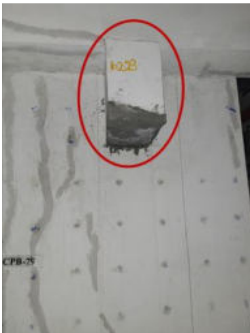
(i) Cosmetic repair of spalled region in corbel and cracks in shear wall and beam
